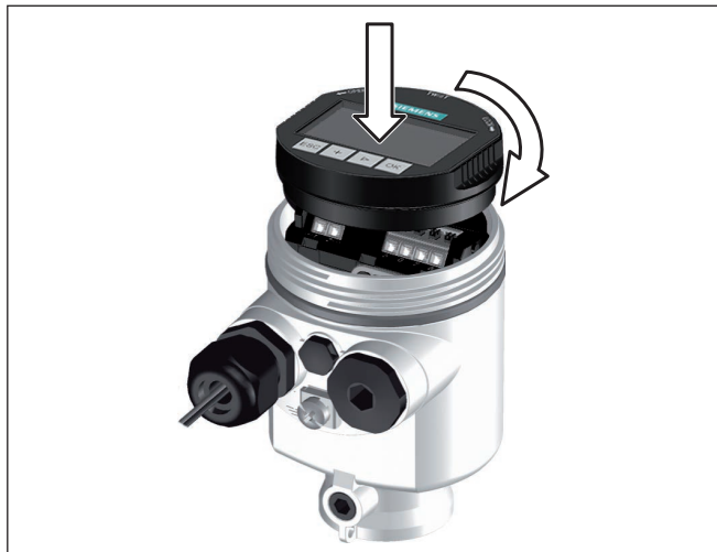
Fig. 13: Insertion of the display and adjustment module with single chamber housing into the electronics compartment
